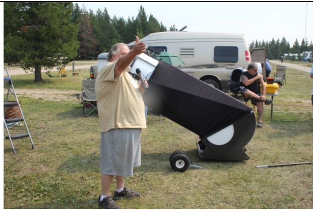
Doug McIntosh showing his computerized 24 inch f/3.3 StarStructure Horizon w/Lockwood mirror, the biggest telescope
