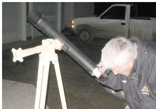
Garry Stone's project for the winter was building a pair of 90mm fibreglass telescopes. Here is one of them, with a homebuilt tripod to go with it.
