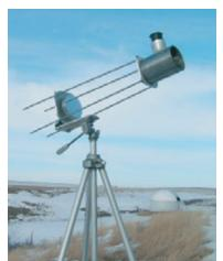
Garry Stone is continuing with his tradition of building a new telescope each winter. Turning aside from fiberglass and wooden refractors, this winter he is working on a Newtonian built out of a surplus three-inch mirror.
